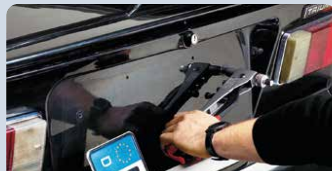
Number plates can be changed with effortless ease thanks to the thread in the rivet nut.
