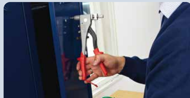
Riveting makes fast work of attaching and changing nameplates. For instance, changing-room lockers can be labelled in a matter of seconds.
